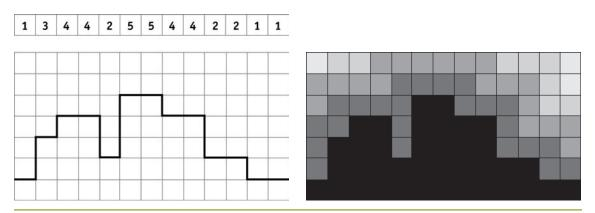
**Figure 8-4.** A Sample Distance Map in Two Dimensions
