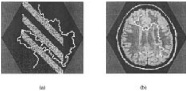
Fig. 5. The user points at two hexagonal spels of the real-valued picture. Based on these, a fuzzy spel affinity is calculated as explained in the text. In both images, the indicated chain is a strongest possible chain (for the calculated fuzzy spel affinity) between the two user-selected spels (it has been generated using a version of Dijkstra's algorithms that also tries to optimize with respect to a secondary criterion, as explained in the text).
