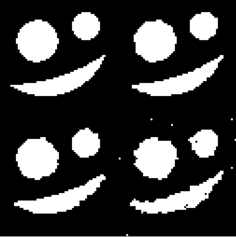
Fig. 6. A phantom (upper left corner) and its reconstructions using noiseless raysums (upper right corner) and raysums with additive noise of mean 0 and standard deviation ( \sigma ) of 0.5 (lower left corner) and 1.0 (lower right corner)
